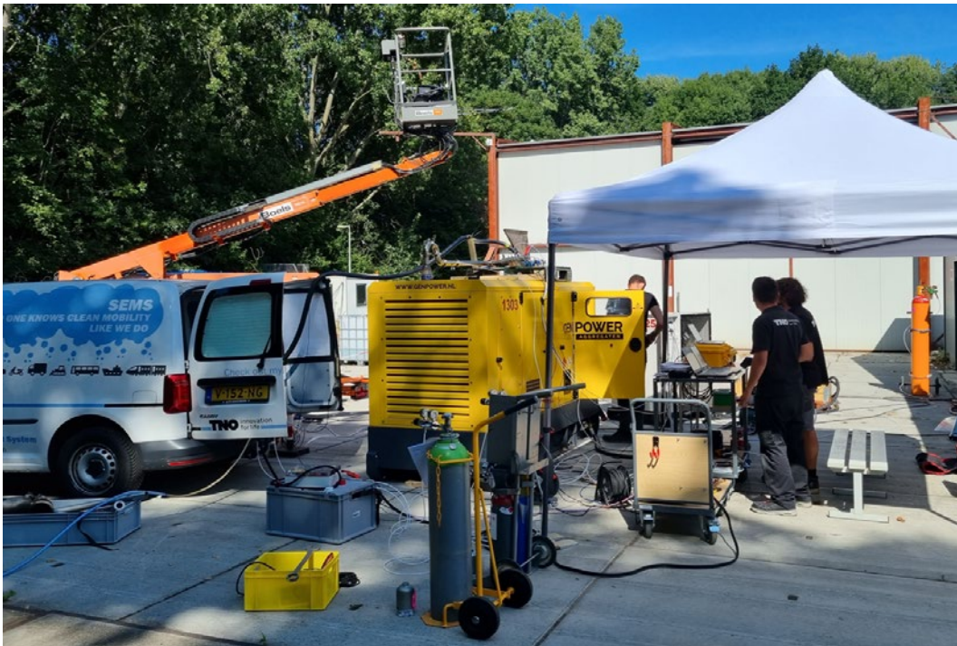
Figure 11. The land-based test with a diesel genset with methane dosage in the exhaust and the drone mounted on a crane.
