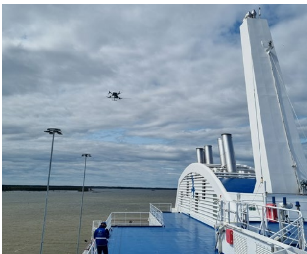
Figure 9. Drone flight measuring \text{CH}_4 , \text{NO}_x and \text{CO}_2 concentrations in the exhaust plume of the Aurora Botnia when only main engine 4 was running. Fuel-fired boilers are switched off. The stacks are the stacks of the four main engines and two fuel-fired boilers. The high funnel in front contains the boil-off and crankcase gas venting pipes.
