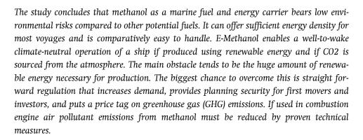
Upscaling the production and supply of RNFBOs is crucial to decarbonize maritime transport. So far, there is little experience using hydrogen, e-methanol or e-ammonia as a fuel in shipping. It is further not yet clear which fuel is the most appropriate for use in deep-sea shipping and which option will gain the highest share in the future fuel mix.
