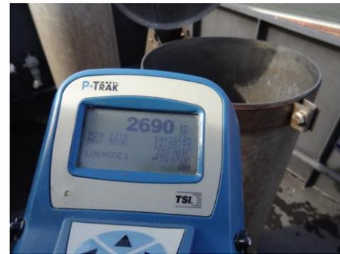
Particulate counter shows very low UFP concentration directly next to the smoke stack.
