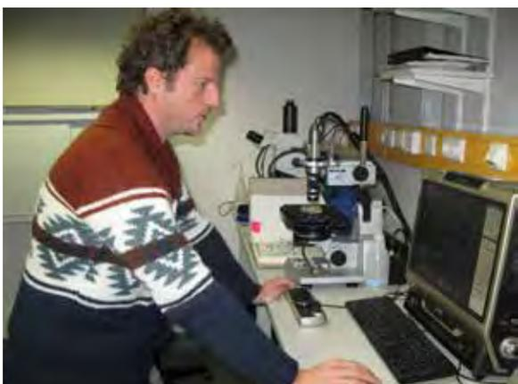
**Figure 30:** Keyence VHX-2000 digital microscope (photo: Thies Geertz)
