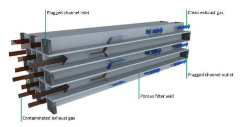
wall flow filter principle
