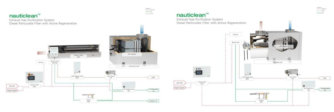
diesel burner for regeneration (burner pipe or chamber) reactor housing with filter cassettes (various aspect ratios)
