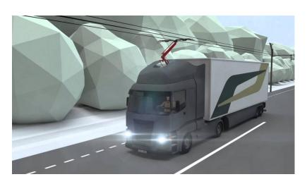
Electrified roads: certain share of the road network to be equipped with overhead wiring (or inductive charging?), driving on the non-electrified parts with battery power or diesel/gas engines. Costs of 2 mio. €/km have been quoted.
