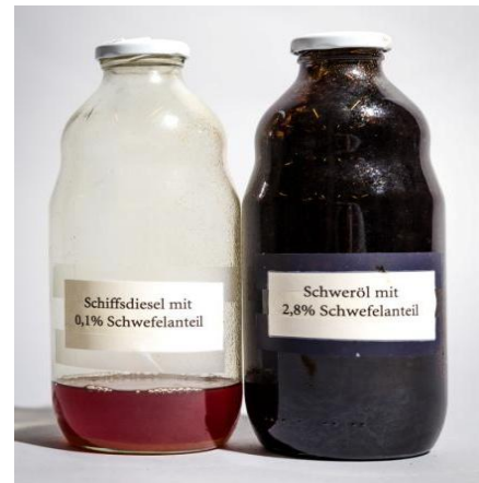
Marine diesel with 0.1% sulphur compared (left) to heavy fuel oil (HFO) 2,8% (right)
